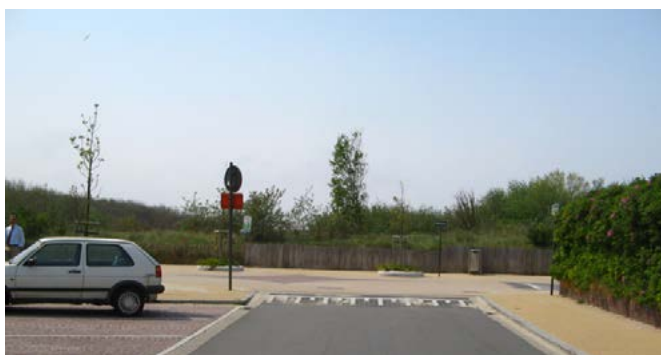
Fig. 7. & 8. Zeebrugge, Belgium. The surface of the intersection is elevated to the level of the pavements and integrated with their surface. Source: photo by Hubert Trammer, May 4 th , 2007.
