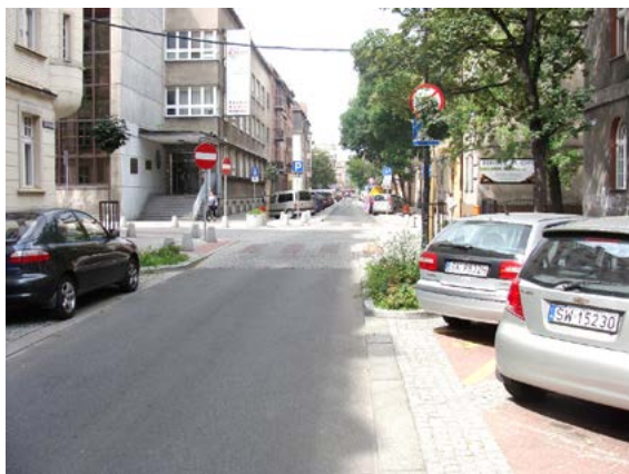
Fig. 5. & 6. Intersection of Juliusza Ligonía St. and Królowej Jadwigi St. in the centre of Katowice. The surface of the intersection is elevated to the level of the pavement and marked by paving. Source: photo by Hubert Trammer, August 3 rd , 2014.
