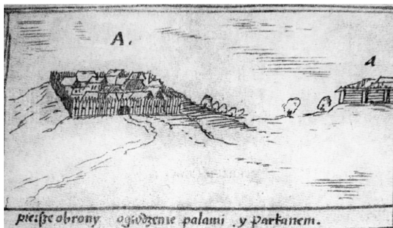
Fig. 5. Two old types of defensive walls of the city, which were built using wooden logs and piles: A – fortifications from sharpened, vertically dug piles; It was built on the top of an earthen rampart (so-called “Tyn”); a – fortifications from horizontal logs and piles (so-called “Fence”); as a rule had loopholes and roof; was built on the top of the earthen rampart (from the treatise by J. Naronowicz-Naroński, 1659 [J. Naronowicz-Naroński, 2016, s. 12]).
