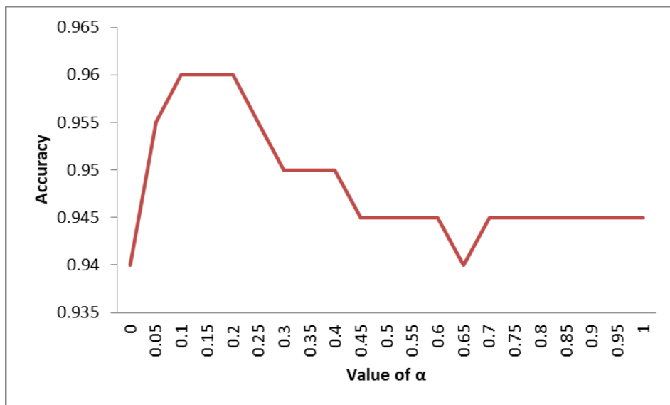
Fig. 5.29 The values of \alpha in relation to the accuracy of the aggregation of various classifiers for the whole face FERET images.
