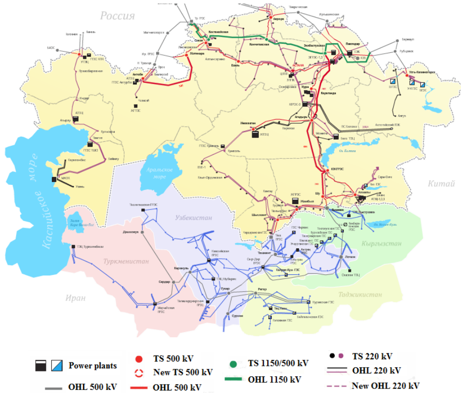
Fig. 4.3. Power grid of Kazakhstan [74]
