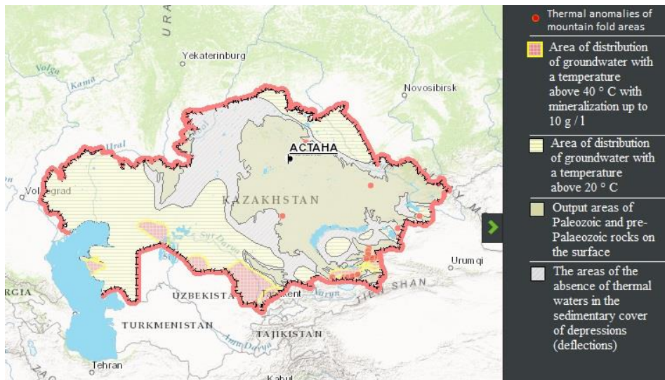
Fig. 5.23. Map of the thermoanomalies and energy potential of hydrogeothermal resources in perspective areas of Kazakhstan [42]
