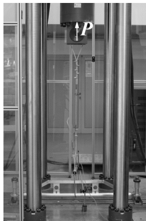
Fig. 4.11 The view of the whole test stand with a ledger loaded by concentrated force applied in mid-span
