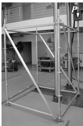
Fig. 4.12 The test set-up to examine load bearing capacity of standards
