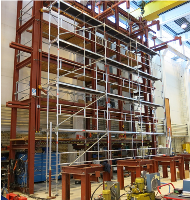
Fig. 4.3 The scaffolding used by the Swedish Technical Research Institute in the global test
