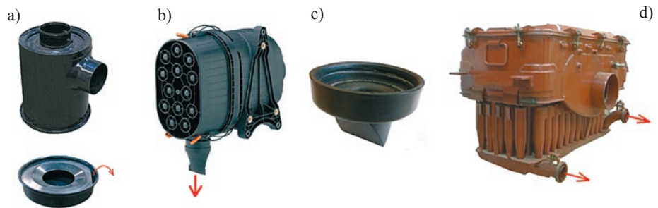
Fig. 4. Dust extraction methods for inertia filters: a) manual (Jelcz 317 filter), b) rubber drain cone (Mann+Hummel filter), c) rubber drain cone d) ejection (T-72 tank filter)
