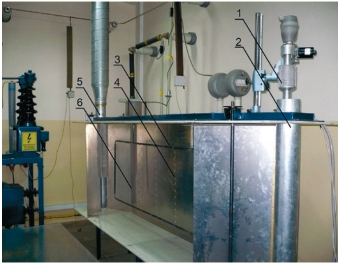
Fig. 4. View of laboratory electrostatic precipitator with removed collecting electrode. 1 – the dust feed system, 2 – diffuser, 3 – frame of discharge electrodes, 4 – discharge electrode, 5 – confuser; 6 – collecting electrode
