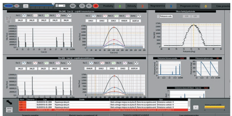
Fig. 12. Application panel with the major technological parameters of the selected forging process
