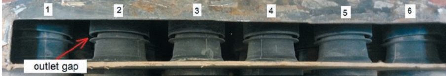
Fig. 16. Cyclone outlet gaps after maintenance – view from the dust extraction manifold: 1, 2, 3, ..., 6 – consecutive cyclone number in the column
