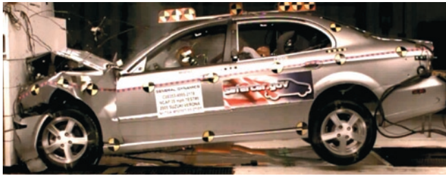
Fig. 4. Frontal impact of a car with a rigid barrier [24]
