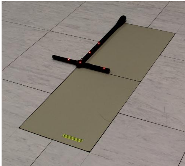
Fig. 1. Arrangements of two force plates [source: own study]
