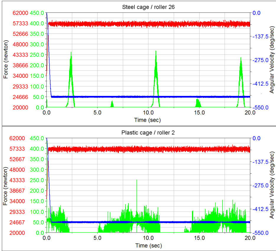
Fig. 4. Force interaction between inner ring and rollers (red lines), force interaction between cage and rollers (green lines) and angular velocity of rollers [source: own study]
