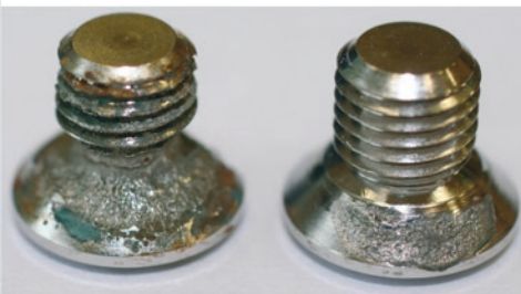
Fig. 8. View of the surface of the POLFIX fastening screw head: a) mag. x30, b) mag. x50
