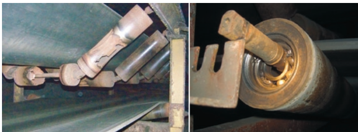
Fig. 9. Examples of premature wear of idlers [10]
