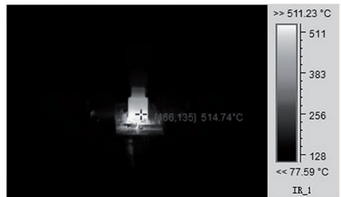
Fig. 3. Infrared image of FSW
