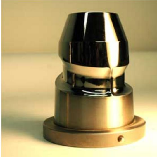
Fig. 11. Example of cylindrical heart-shaped mandrels with a visible manifold (Guill Tool & Engineering USA)
