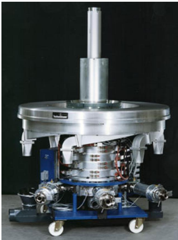
Fig. 24. Transverse extrusion head for blown film with an internal film cooling system and an external cooling ring (Reifenhäuser Extrusion, Germany)
