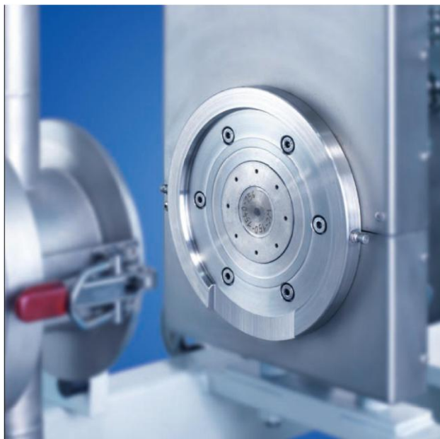
Fig. 36. Ending of the extrusion head for hot pelletizing in water (Econ-Kundenberatung, Austria)
