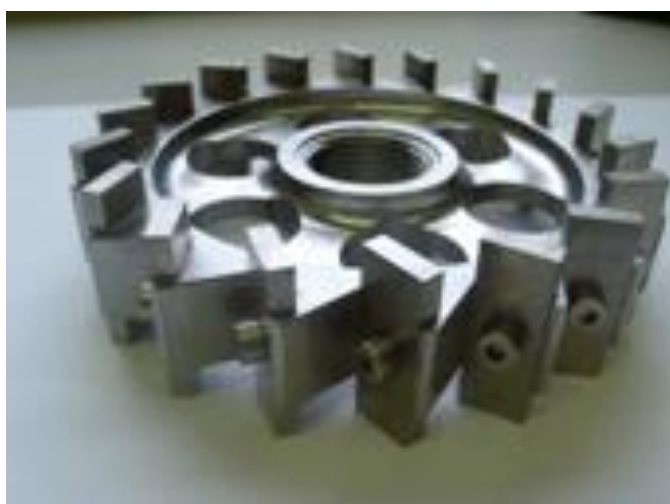
Fig. 38. Pelletizer rotor with cutting blades (Kreyenborg Granulierteknik, Germany)
