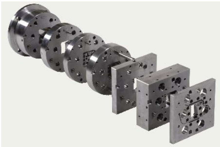
Fig. 22. Specific components of the longitudinal multi-plate extrusion head (Greiner Extrusion, Austria)
