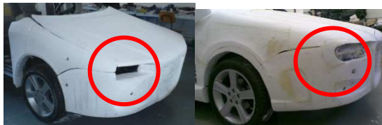
Fig. 20. Prototype of the bumper before (left) and after the adjustments
