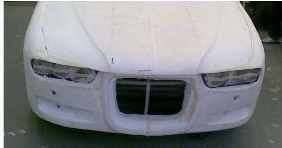
Fig. 21. Finished polystyrene model of the bumper
