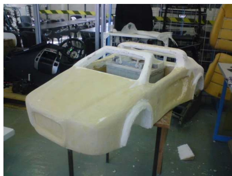
Fig. 7. Mockup fabrication (scale 1:4)
