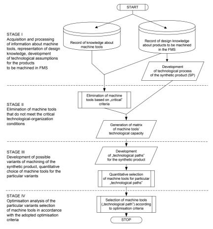
Fig.1. Main algorithm of the methodology of machine tools selection in casing-class FMS [9,19]
