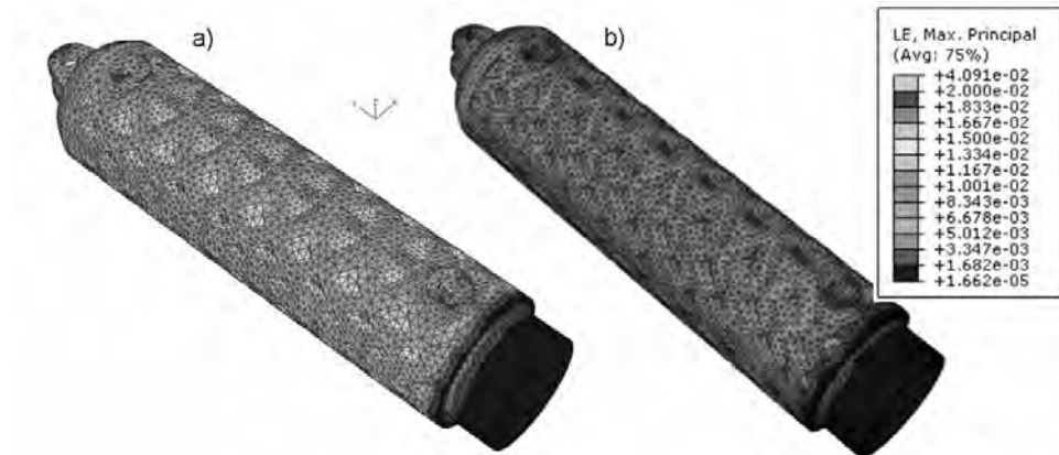
Fig. 9. Deformation maps for a pneumatic servo body: a) orthotropic model, b) isotropic model
