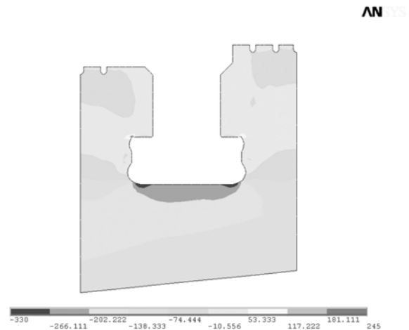
Fig. 12. Distribution of the axial stresses at point A in the blade groove in the 107 th minute of the start-up from the cold condition
