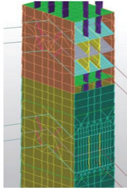
Figure 4.4.14. Section through the pylon of a bridge of Solidarity (by MJ)
