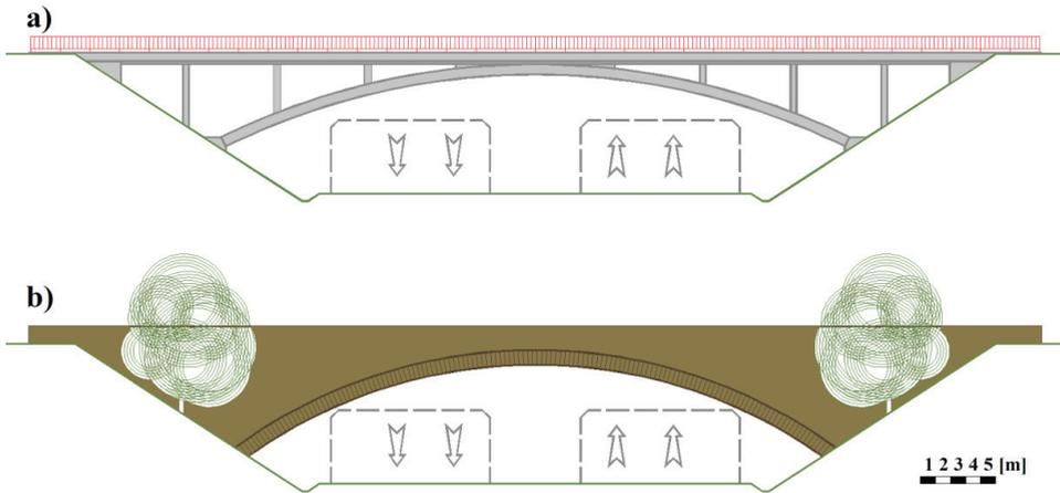
Figure 4.1.1. One span arch viaducts a) openwork, b) solid
