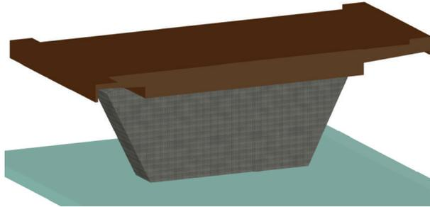
Figure 4.4.8. Pillar riverine with the front inclined towards the foundation (*by MJ*)
