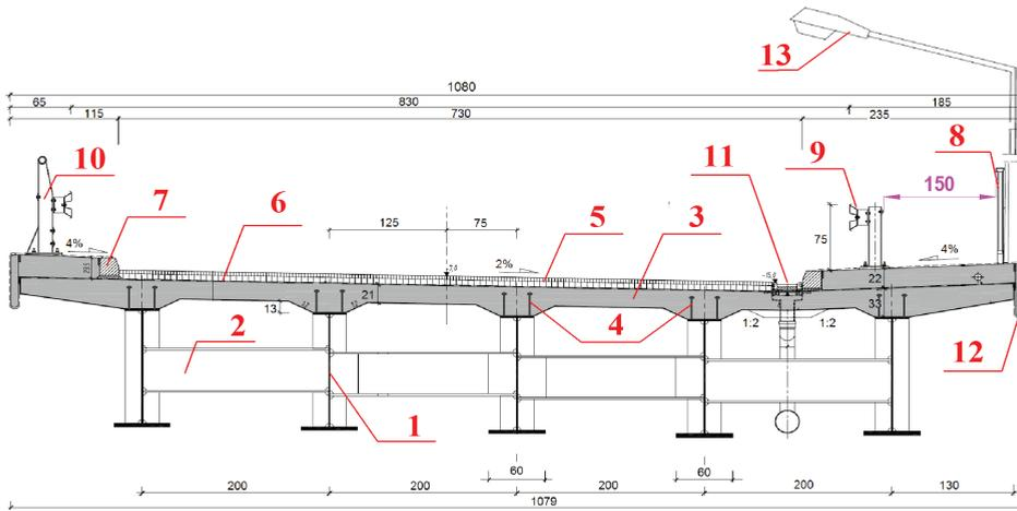
Figure 7.5. The cross-section of composite highway bridge <sup>129</sup>
