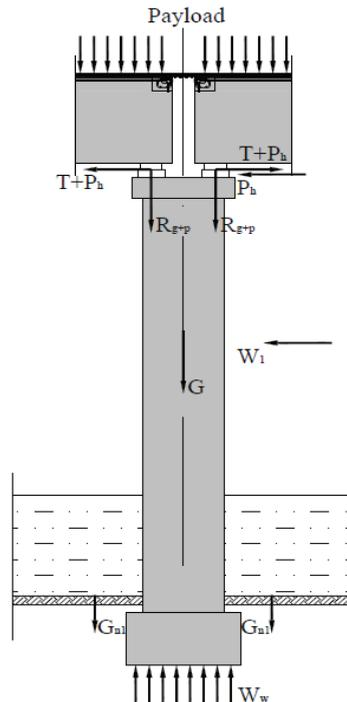
Figure 4.4.12. The forces acting on an intermediate pillar (by MJ)
