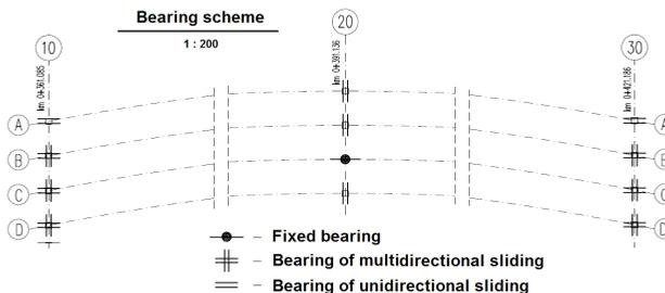
Figure 7.8. The example of bearing in case of three span road bridge <sup>129</sup>
