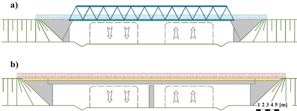
Figure 4.1.4. Viaduct: a) one span truss, b) two span continuous beam
