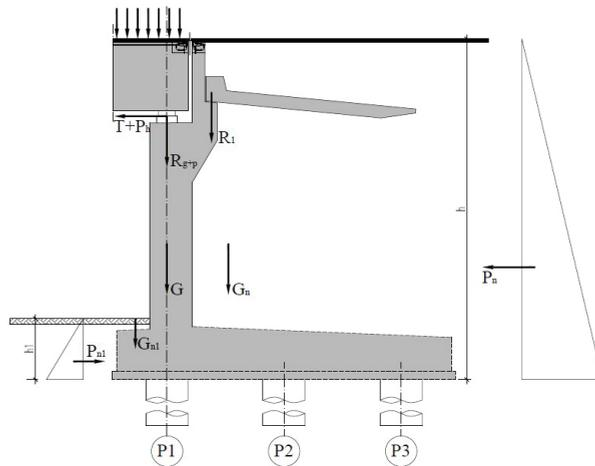
Figure 4.4.4. Forces acting on the abutment when the load is on span bridge (by MJ)
