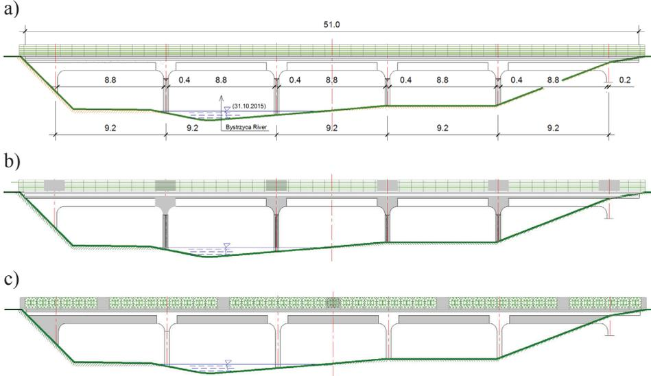
Figure 4.5.4. Possible revitalizing actions of the First Lutoslawski Bridge a) current view b) pilastring c) anti-pilastring
