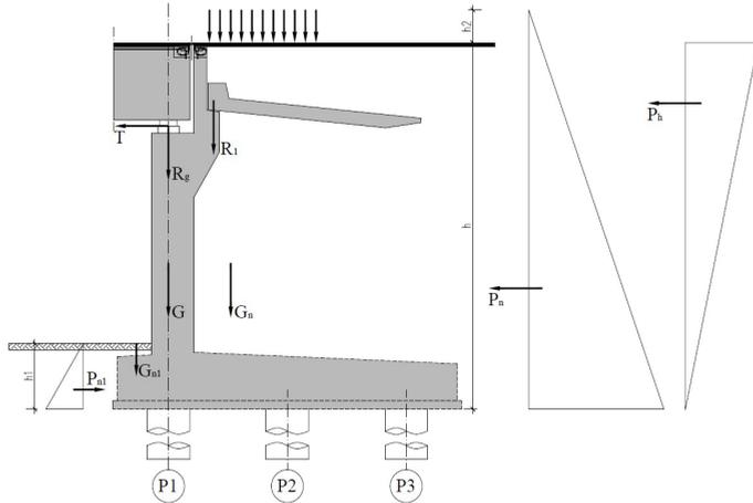
Figure 4.4.3. Forces acting on the abutment when the load is in a wedge fraction (by MJ)
