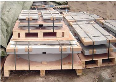
**Spherical bearings.** The storage of modern steel-neoprene bearings for a large bridge. Between steel spherical members the PTFE strips are placed. Also in this case one can distinguish the bottom and upper plates as well as the bearing element.
