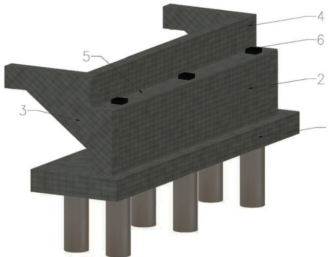
Figure 4.4.2. Structural elements of abutment brak numerów (by MJ)
