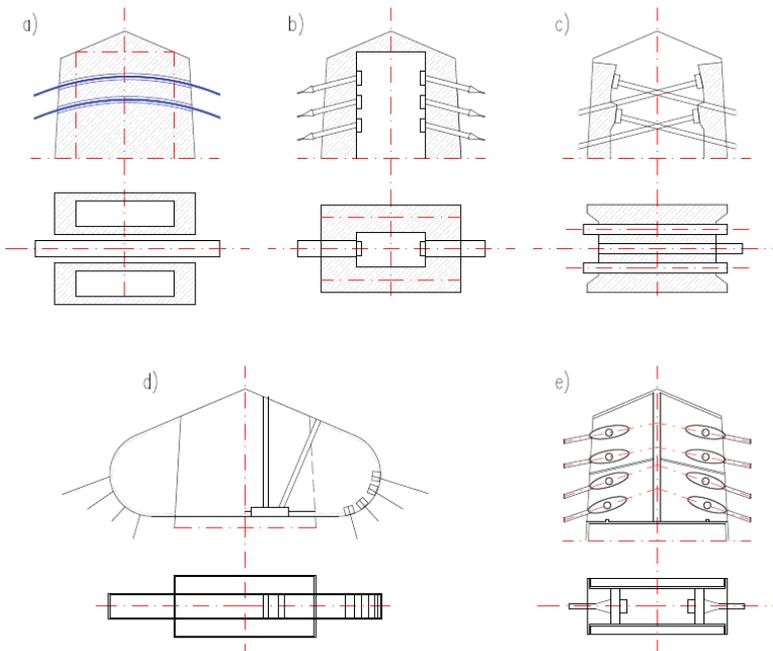
Figure 4.4.13. Different ways of attaching the suspension rods to the structure of the pylon (by MJ)
