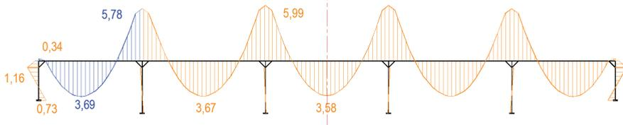
Figure 4.5.2. The frame static scheme of the first Lutoslawski bridge in Lublin a) Load – [kN/m] and geometry [m] b) Bending moments for existing bridge scheme, [kNm] c) Frame with reduced extreme span lengths, bending moments [kNm]
