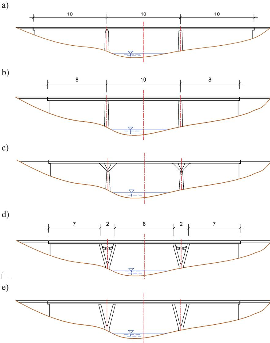
Figure 4.5.1. Study of 3 span bridge a) 3 simple span beams b) continuous beam c) caddles on verticals d) additional bracing in V pillars e) V shape of pillars only
