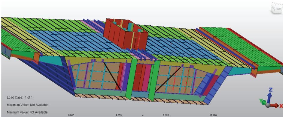
Figure 4.4.15. View of the connection the pylon of the span (by MJ)
