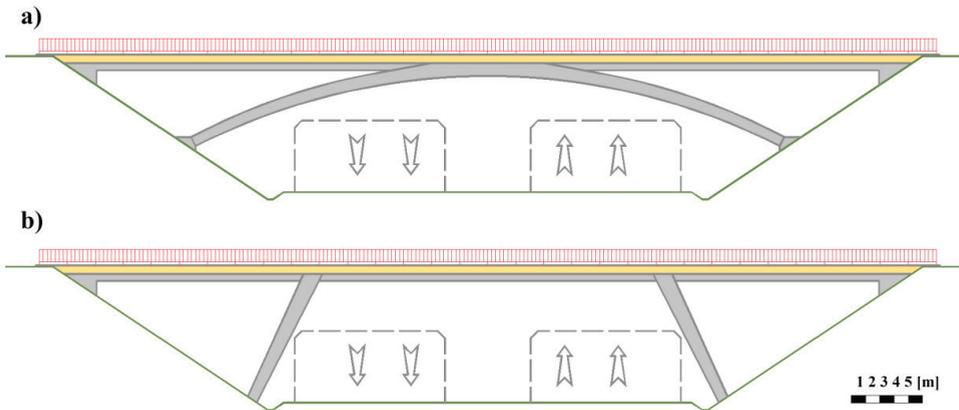
Figure 4.1.3. Three span frame viaducts: a) derived from arch, b) simple
