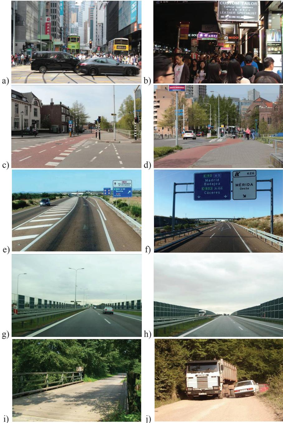
Figure 3.2.1. Road arrangement a–b) big city traffic (HK) c–d) vertical and horizontal markings on a street (NL) e–f) markings on the expressway (ES) g–h) noise screens on an expressway (PL) i–j) country roads (PL); (a–d photos by Paulina Jaminska)
