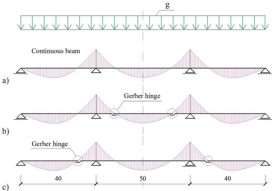
Figure 7.1. The Gerber concept of a hinge system a) the graph of bending moments in the case of a uniformly loaded continuous beam b) 1<sup>st</sup> option of hinge distribution c) 2<sup>nd</sup> option (by SLK)
