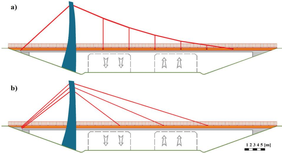
Figure 4.1.5. Viaduct: a) suspension structure, b) cable-stayed structure
