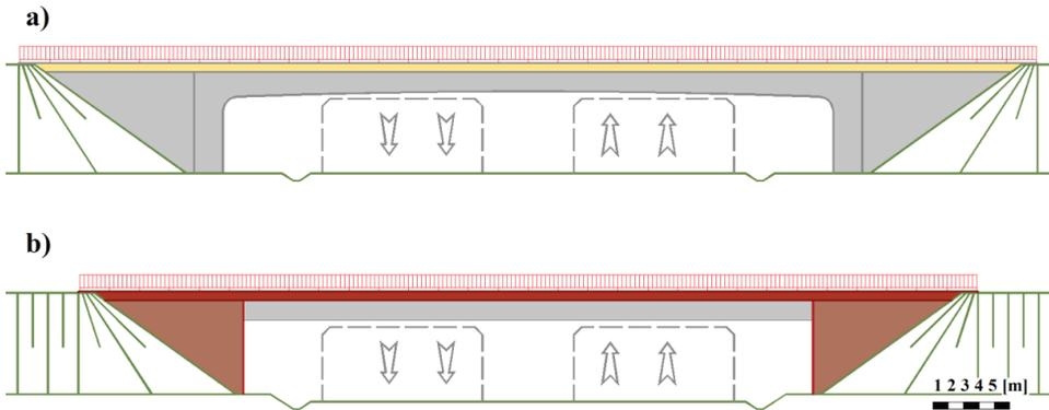
Figure 4.1.2. One span viaducts: a) frame, b) simple supported light beam
