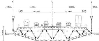
**Izmit Suspension bridge.** Izmit Bay Suspension Bridge – the cross-section of low profile orthotropic bridge deck.
