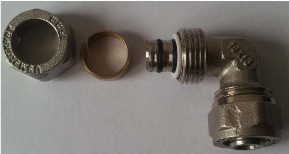
Fig. 1. Picture of tested short DN 16 90 degree elbow
